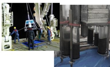
**Figure 7** Multiple corer and sediment cores
