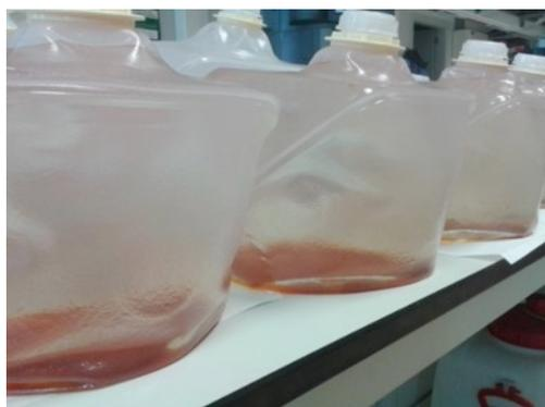
Figure 1: Initial Fe precipitation to extract Uranium isotopes from
