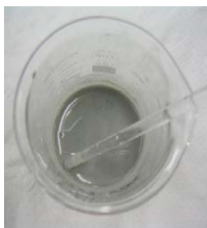
Figure 4 Dissolve AMP/Cs compound by adding alkali solution at step 14
