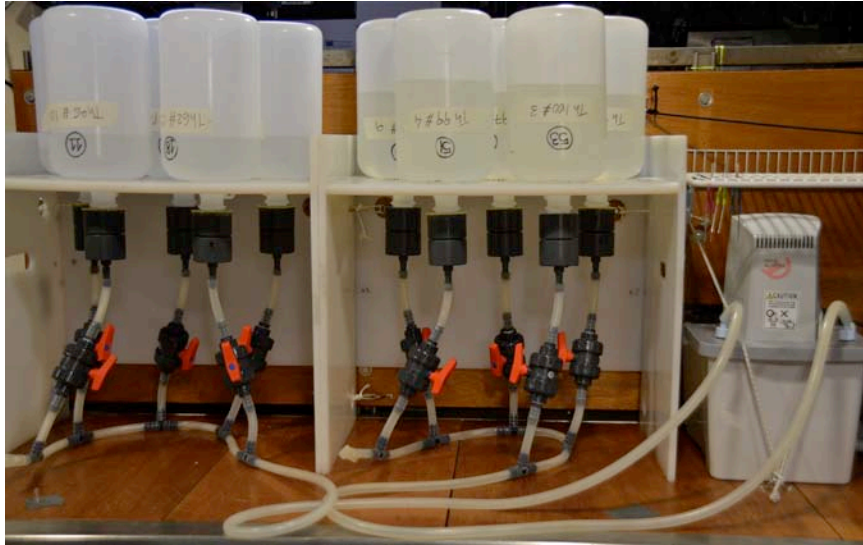
Image 1: Filtration system, with the 4 L bottles containing the sample after being precipitated with MnO_2
