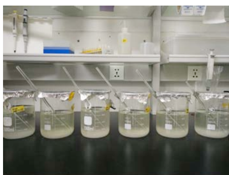
Image 3. Co-precipitation of Ra by \text{BaSO}_4 .
