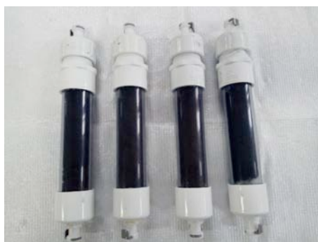
Image 1. Ra in water samples extracted onto Mn-fibers.
