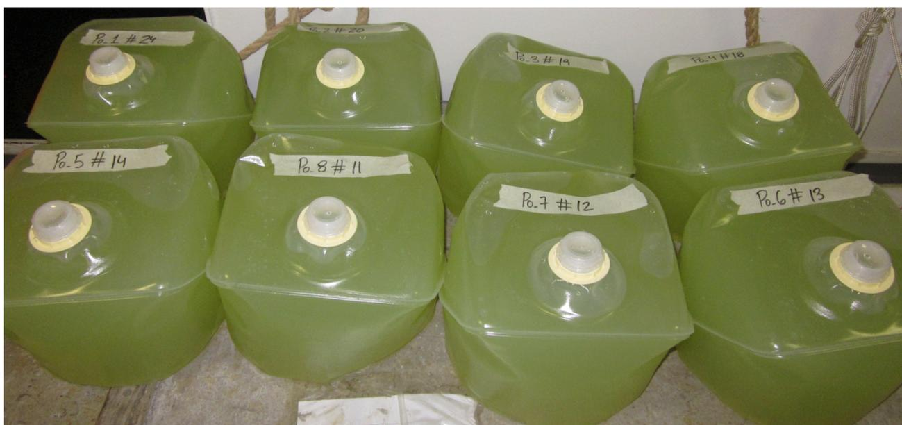
**Image 1:** Samples containing the Co-APDC precipitate (see the yellow-greenish color of the samples).
