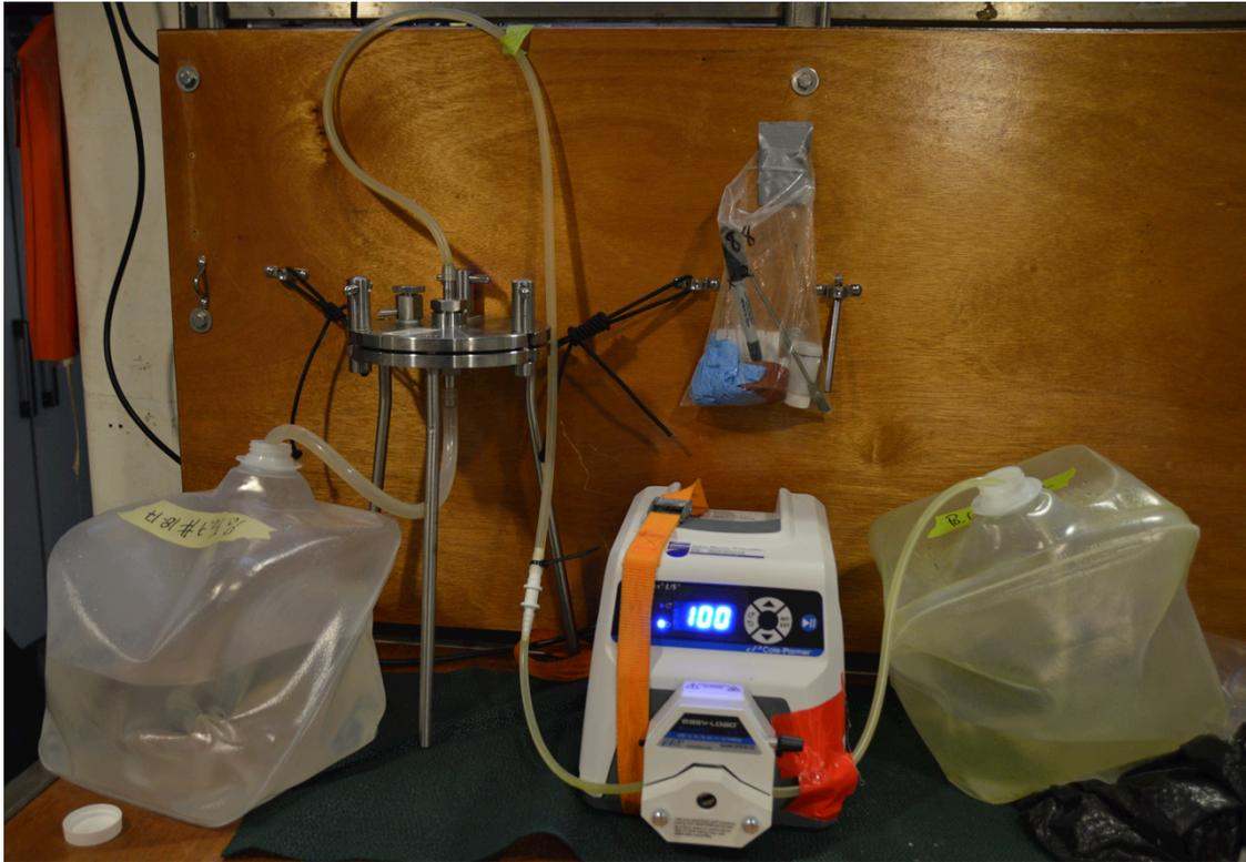
**Image 2:** Filtering the Co-APDC precipitate (right container) through the membrane filter placed on the filter plate using a peristaltic pump. The filtrated (pH <2) is collected on a “waste” container (left container).
